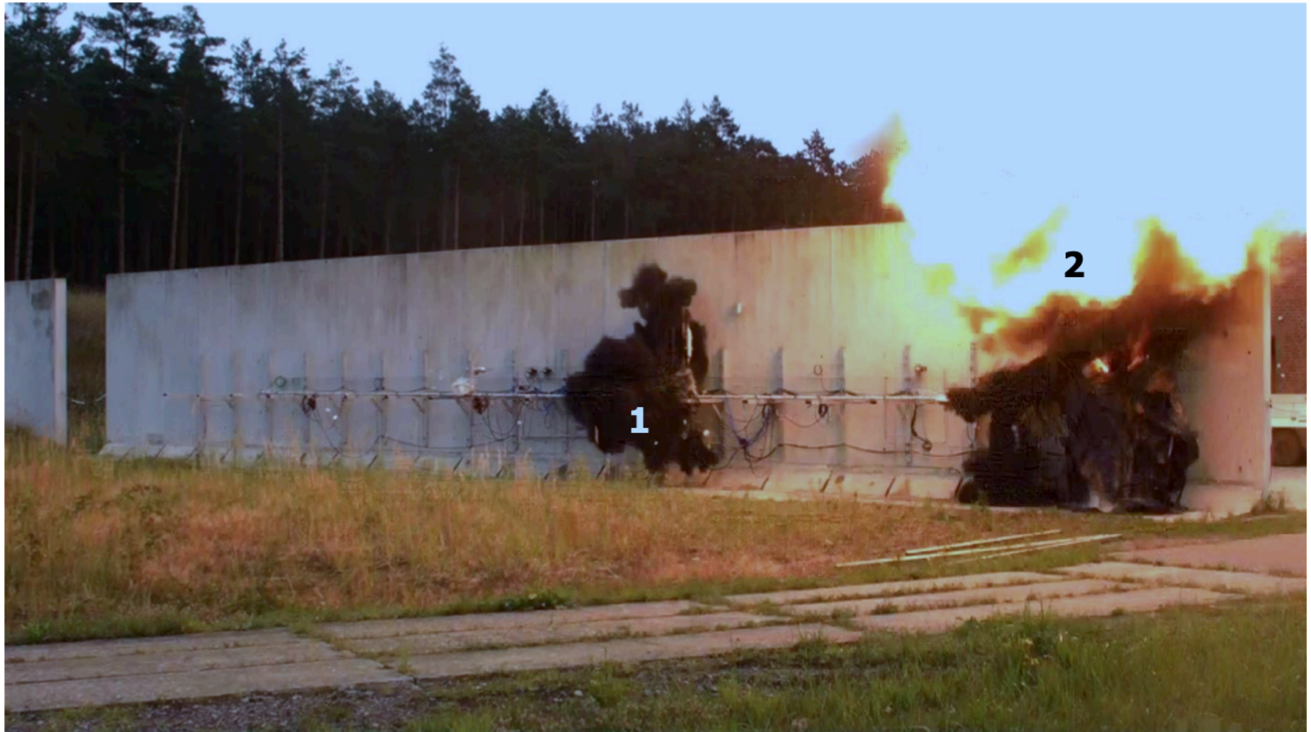
Figure 8 – Picture shot during an ignition of TFE induced by adiabatic compression of air in a large scale facility
