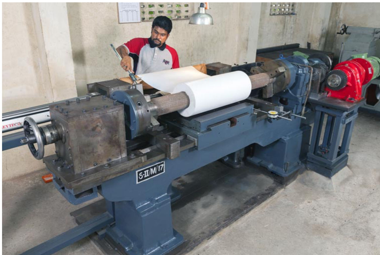
Peeling of film from solid PTFE
