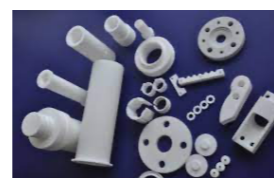
PTFE parts (Bearings, tubes, and seals)
